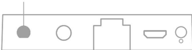
Connect your Flic IR Accessory to the Flic Hub via the 2.5mm connector and place the IR blaster, in the direction of the receiving device(s).
