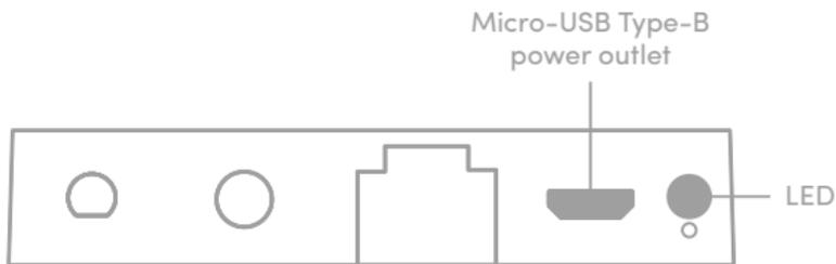
Connect the Micro USB cable and an external power adapter to the Flic Hub. The Flic Hub will turn on, indicated by a bright red LED.
