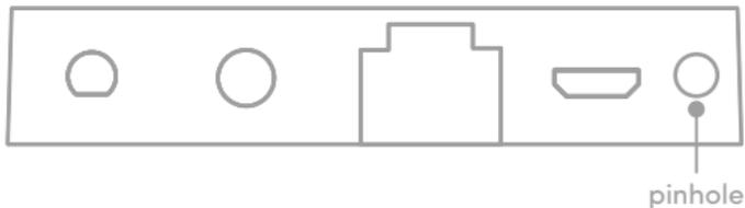
If, for any reason, you must perform a factory reset you need to press the pinhole button for between 10-15 seconds. By pushing the button, all your account settings will be lost and the Flic Hub will return to default.
