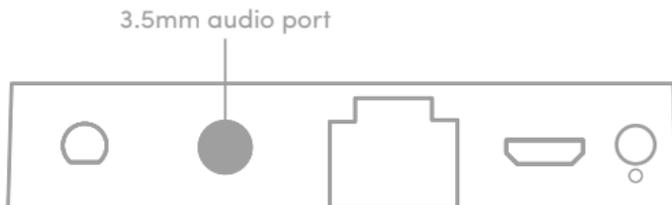
Connect any speaker to the Flic Hub via the 3.5mm audio jack connector.
